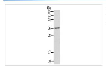
Gel: 10%SDS-PAGE, Lysate: 40  $\pm$ Og, Lane: Mouse liver tissue, Primary antibody:47490(UBXN2A Antibody) at dilution 1/200, Secondary antibody: Goat anti rabbit IgG at 1/8000 dilution, Exposure time: 10 seconds
